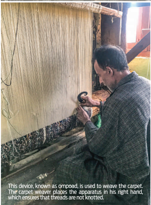
The initial step in the carpet-weaving process is to hang the thread, known as yeoni pan in Kashmiri, in the logs of wood. Two large logs of wood are used. On the top of the wood, threads of several colours are connected.
