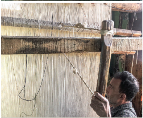
The wooden block has been renamed as kamaan , and it is used to loosen or tighten the carpet. It is attached to a wooden block with a rope-like thread that the weaver created himself. After then, it is pushed back and forth.
