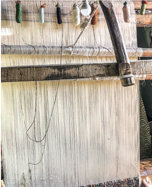
The initial step in the carpet-weaving process is to hang the thread, known as yeoni pan in Kashmiri, in the logs of wood. Two large logs of wood are used. On the top of the wood, threads of several colours are connected.
